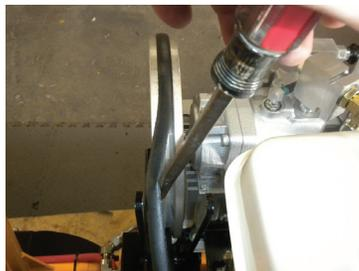
4. Insert screw driver between belt and large pulley.
