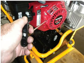
5. Pull starter rope until belt get off pulley.
