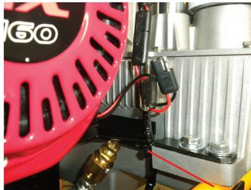
6. Disconnect electric wire connection that go to engine only, and then cut off tie (mark red).
