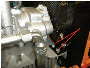
3. Open the 2 bolt and remove cover to expose belts.
