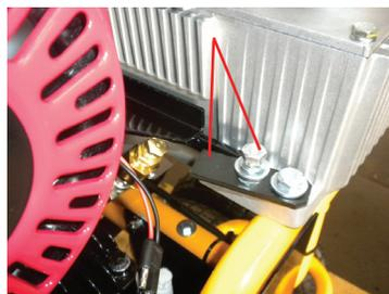
7. Open bolts move the bracket to the side, then lift engine and remove it from belts.
