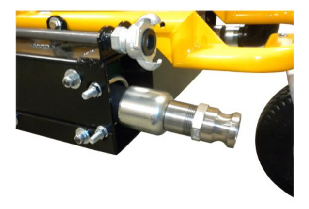
All Benron squeeze pump material hoses include a special internal expansion fitting on the outlet hose connector, that allows material to flow without any friction due to a smooth and easy transition from the squeeze pump hose to the material hose.
