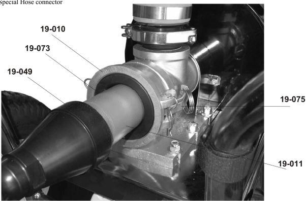
**Note:** To remove stator for cleaning purpose, remove safety pins and open locks.
