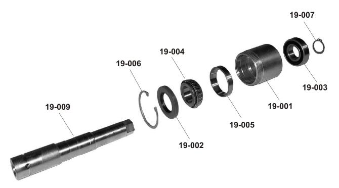
**Note:** Pack bearing with heavy duty marine grease.
