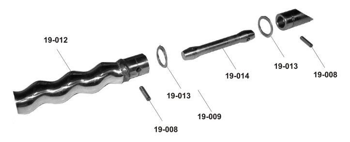
**Note:** Inspect parts 19-008 and 19-014 if found worn out parts must be replaced.
