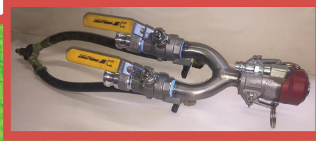
Spray gun with solvent port clean-out
