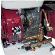
**Note: If pump is seized, insert tool provided to free rotor in the hole at the center of the belt guard and cover as shown below. Now turn until rotor feels free. You must remove tool before starting the sprayer.**
